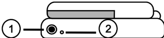
3. The LED stops blinking and glows a steady green once the batteries are charged. Unplug the power adapter from RUBY. The battery indicator LED turns off.
